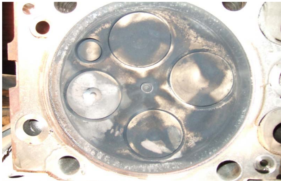
Photo 8. Cylinder cover of Mercedes-Benz reg. no 062 ARU at operation with diesel fuel with catalyst MPG -MEGA – Crumbs™.
